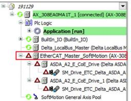
3. To restore the network connection between the master and the slave, shift the input bExecute of DFB\_ResetECATMaster to True.
