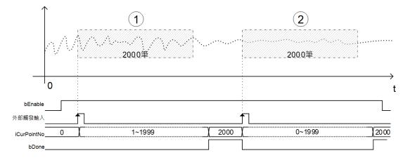
The fixed period + trigger start mode is similar to the fixed period mode, but the recording start timing of the fixed period
