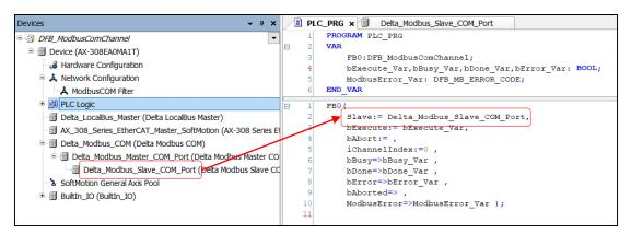
\*Note: The input of Slave would be the name of Modbus slave device.
