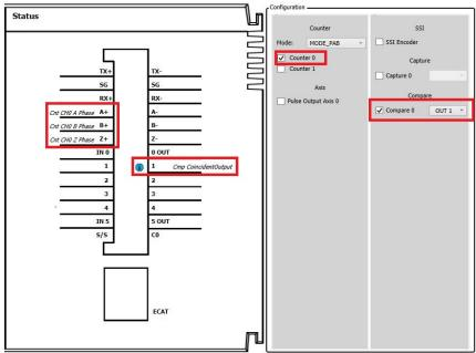
Execute the function block DFB\_Compare after enable the high-speed counter by using DFB\_HCnt in the POU as shown in follows. At the same time, the output device (OUT1) will output the signal once the comparison condition is fulfilled (DFB\_HCnt\_0.diCounterValue = DFB\_Compare\_0.diCmpValue).
