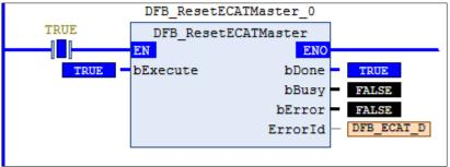
4. The network connectivity has been recovered after the output bDone shifting to True.
