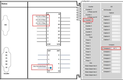
2. Execute the function block DFB\_Compare after enable the high-speed counter by using DFB\_HCnt in the POU as
