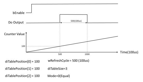
OutputAction is an output variable that define the action of the output device once the comparison condition is met. When it is set to SET, the output device will be set to high level. When it is set to RESET, the output device will be set to low level.
