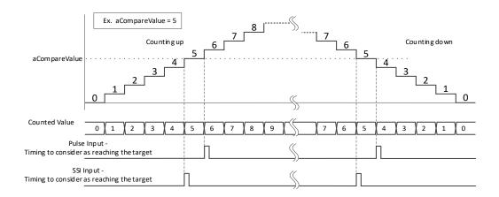
Take **aCompareValue** = 5 as an example, SSI input compare arrival timing occurs in the counter value  $4\rightarrow 5$  and  $6\rightarrow 5$  instantaneous. For pulse input, when counting up, compare arrival timing occurs in the counter value  $5\rightarrow 6$  instantaneous; when counting down, compare arrival timing occurs in the counter value  $5\rightarrow 4$  instantaneous.
