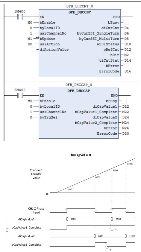
\* 1: bCap Value1\_Complete is not cleared to OFF, the captured value still up dates in di CapValue 1. \*2: bCap Value2\_Complete is cleared to OFF, the captured value still up dates in CapValue 2.
