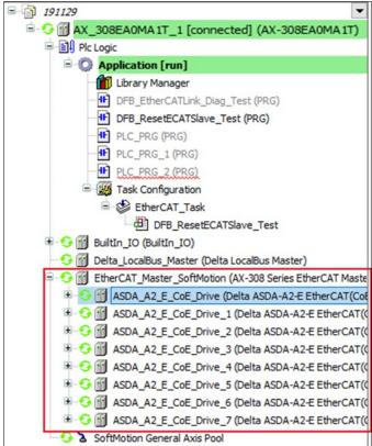
2. Remove the network connection of slave 4 and 5, and the current connection status of EtherCAT slave starting from slave 5 would show Fail in the device tree.
