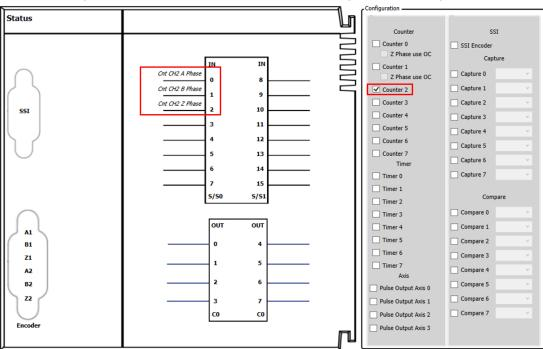
2. After using the FB DFB\_HCnt in the POU to activate the high-speed counter(bEnable = True), it starts receiving and counting the pulses from the external signals(IN 0, IN 1) based on the counting mode set in Counter Configuration, then the counter value would be displayed in the output diCounterValue. In addition, you should make sure that the mode of sending pulses from the external signal source matches the counting mode so as to get the correct counter values.
