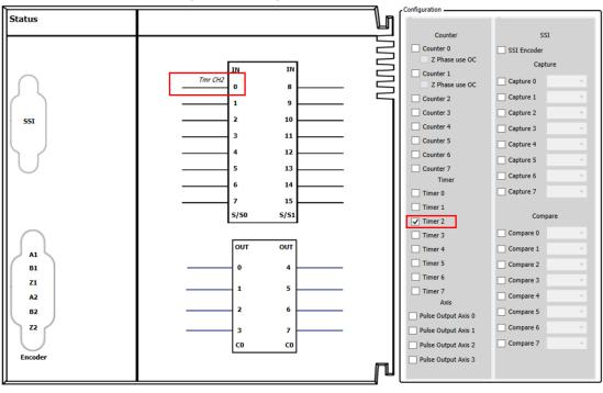
After using the FB DFB\_HTmr in the POU to activate the high-speed timer(bEnable = True), it starts receiving and counting the pulses from the external signals(IN 0) based on the timing mode set in Timer Configuration, then the timed value would be displayed in the output dwTimerValue.
