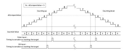
Take **diCompareValue** = 5 as an example, SSI input compare arrival timing occurs in the counter value  $4\rightarrow 5$  and  $6\rightarrow 5$  instantaneous. For pulse input, when counting up, compare arrival timing occurs in the counter value  $5\rightarrow 6$  instantaneous; when counting down, compare arrival timing occurs in the counter value  $5\rightarrow 4$  instantaneous.
