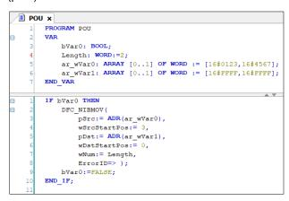
Since wSrcStartPos=3, wNum=2 and wDstStartPos=0, two consecutive Nibbles (Length=2), which start from Nibble3 of variable ar\_wVar0 (pSrc), are shifted to the address Nibble0 inside the memory of ar\_wVar1 (pDst).
