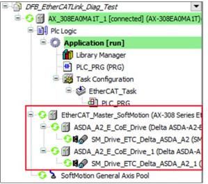
After bEnable of DFB\_EtherCATLink\_Diag shifts to True, the output uSlave shows 2, indicating that there are two EtherCAT slaves in total. The array of StationNode index 1 to 2 shows the two slave addresses, statuses, and physical connection statuses, and the StationAddress of StationNode shows 0 from index 3.
