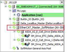
2. Remove the network connection between the master and the slave, and the current connection status of EtherCAT master would show Fail in the device tree.
