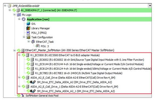
2. After the input bExecute of DFB\_EcGetAllSlaveAddr bExecute shifts to True, the output of AddrArray is shown as below and the output value of uSlaves is 7.
