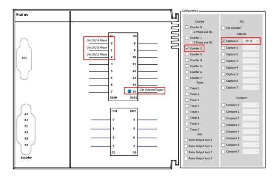
Enable the FB DFB\_Capture (bEnable = True) after using the FB DFB\_HCnt to activate the high-speed counter (bEnable = True) in the POU, then the present counter value would be captured and shown on the diCapValue output of DFB\_Capture after the external signal (IN15) being triggered.
