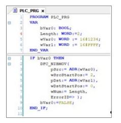
Since wSrcStartPos=2, wNum=2 and wDstStartPos=0, two consecutive Nibbles (Length=2), which start from Nibble2 of variable wVar0 (pSrc), are shifted to the address Nibble0 inside the memory of wVar1 (pDst).
