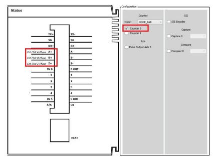
2. After using the FB DFB\_HCnt in the POU to activate the high-speed counter(bEnable = True), it starts receiving and counting the pulses from the external signals(A+A-/B+B-) based on the counting mode set in Counter Configuration, then the counter value would be displayed in the output diCounterValue. In addition, you should make sure that the mode of sending pulses from the external signal source matches the counting mode so as to get the correct counter values.
