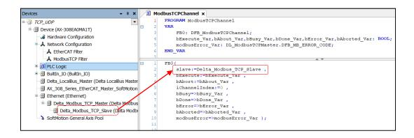
\*Note: The input of Slave would be the name of Delta\_Modbus\_TCP\_Slave device.
