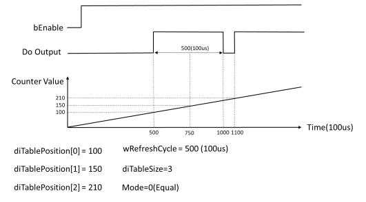
Case2: When comparing multiple values of diTablePosion at the same time, the defined Do output time is the time of of one cycle of wRefreshCycle. Refer the following diagram for the timing and parameter:
