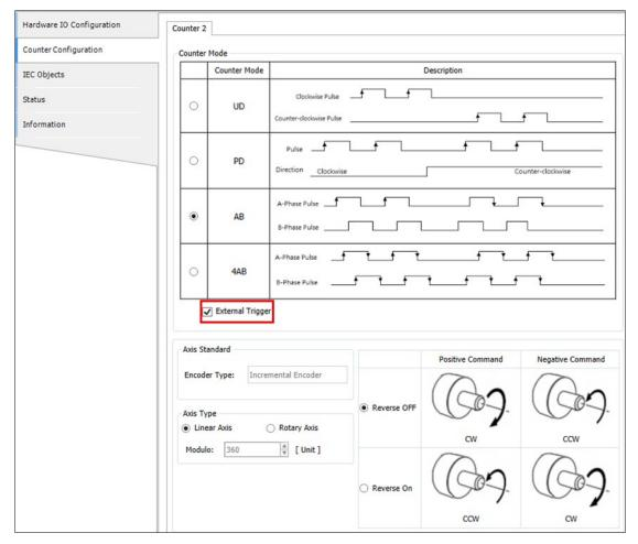
4. Then the input bExecute of DFB\_PresetValue shifts to True and the FB DFB\_PresetValue would wait for the Z phase of high-speed counter to trigger the Default value function. After the counter value being set to the default (DFB\_HCnt.diCounterValue = fb), the output bDone will shift from False to True.
