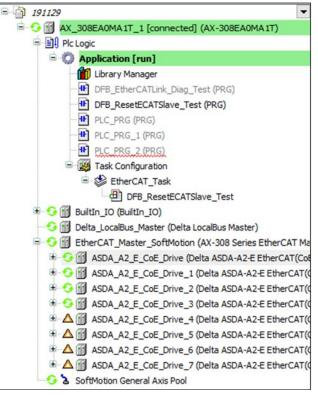
3. To restore the network connection of slave 4 and 5, enter 1005 to the input uiSlaveAddr and shift the input bExecute to True.
