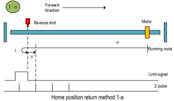
b. Start the home position return → reverse limit valid → Search for the falling edge of reverse limit at low speed forward direction → search for Z pulse in forward direction.
