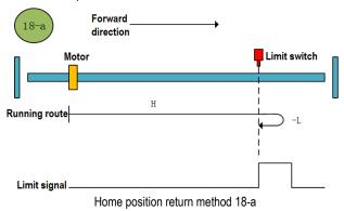
b.Start the home position return  $\rightarrow$ Forward limit valid  $\rightarrow$ Stop after searching for the falling edge of forward limit at low speed reverse direction.
