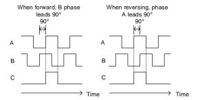
Parameter Pn072 can be set to revert the logic of the AB phase signal of the divided output pulse.
