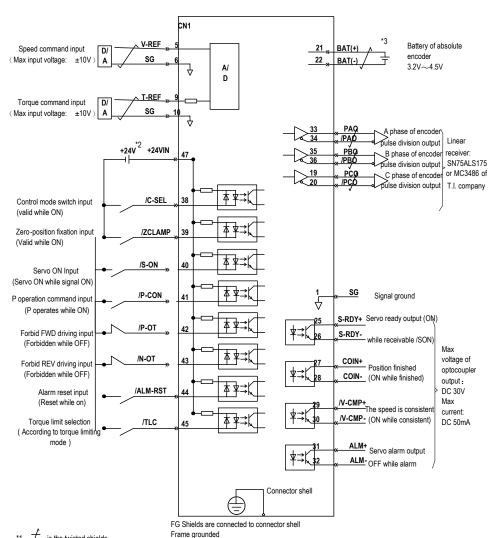
is the twisted shields. \*2. DČ24V power should be prepared by user. And double insulation or reinforced insulation equipments should be used for DC24V power.
