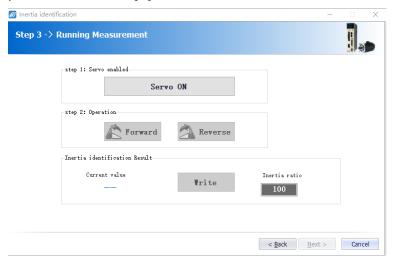
c). Click [Write]→[Next]→[Complete] to finish the inertia recognition process.
