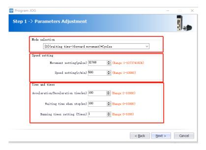
b). After setting the corresponding parameters, click on [Next]  $\rightarrow$  [Write]  $\rightarrow$  [Enable]  $\rightarrow$  [Execution]  $\rightarrow$  [Next]  $\rightarrow$  [Complete]. The program JOG operation process ends.
