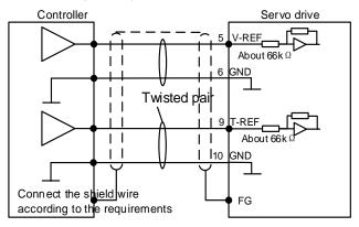
The above wiring is an example of wiring during forward rotation.
