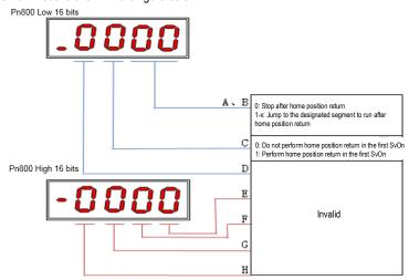
As shown in the figure above, section C of Pn800 is defined as home position return automatically trigger when power on. When the C segment is set to 1, it performs the home position return automatically when the servo is enabled for the first time.
