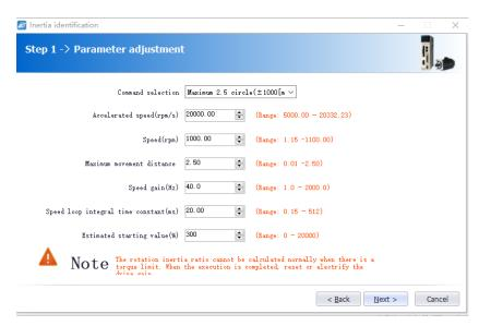
b). As shown in the above figure, set the corresponding parameters according to the actual situation (usually keep the default), and click [Next]  $\rightarrow$  [Write]  $\rightarrow$  [Next]  $\rightarrow$  [Enable]  $\rightarrow$  [Forward]  $\rightarrow$  [Reverse] After the forward rotation is repeated three times, the final inertia identification result is displayed, as shown in the following figure.
