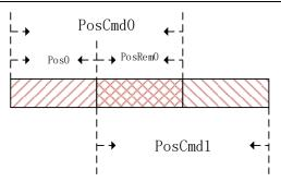
As shown in the figure above, the first position command setting value is PosCmd0. After the pulse of Pos0 is run, the operation ends and the remaining PosRem0 pulses are not completed. If the second relative position command PosCmd1 is inserted at this time, the total number of pulses of the second position command operation is PosCmd1. That is, the second relative position value PosCmd1 is the reference point of the actual position Pos0, and the final running position value is Pos0 + PosCmd1.
