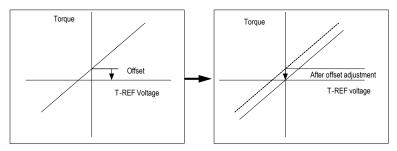
There are two methods of automatic adjustment and manual adjustment of offset adjustment. Automatic adjustment is automatically adjusting the command offset (Fn100) and manual adjustment is manually adjusting using command offset (Fn102). For details, see "Auxiliary Functions".
