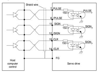
The differential pulse input signal voltage is  $\pm 3.3$ V and the maximum frequency is 4MHz. This signal transmission method has the best anti-noise capability. It is recommended to use this connection preferentially.
