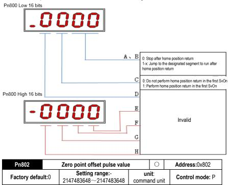
Parameter description: The pulse offset value that needs to be run after the home position signal is found during the home position return process.
