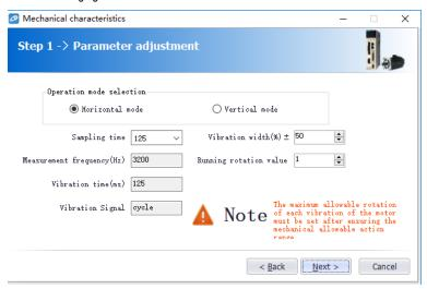
b). Click [Next] → [Write] → [Next] → [Enable] → [Forward] → [Enable] → [Reverse] → [Next] → [Complete] to enter the mechanical properties FFT analysis interface, as shown in the figure below:
