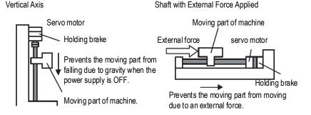
The brake has the following operation delay time. ON and OFF of the operation, please ensure the brake operation time.
