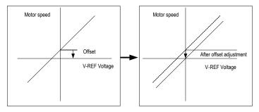
There are two methods of automatic adjustment and manual adjustment of offset adjustment. Automatic adjustment is automatic adjusting command offset (Fn100) and manual adjustment is manually adjusting command offset (Fn101). For details, see "Auxiliary Functions".
