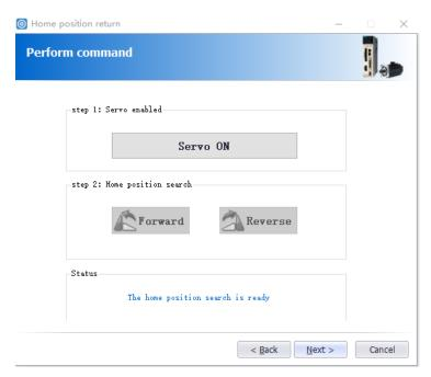
b). Click [Enable] to enable the servo motor to enter the enable state, and then click [Forward Run] or [Reverse Run] to perform the origin search. After the search is completed, click [Next] to enter the back to origin setting interface and click [Completed] to return to origin operation.
