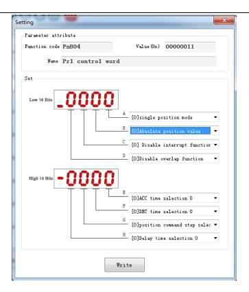
Function code A part function definition: select internal position mode.
