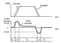
When the switching condition of the mode switch is set as speed command, if the speed command exceeds the speed set in Pn133, the speed loop will be switched to P control.
