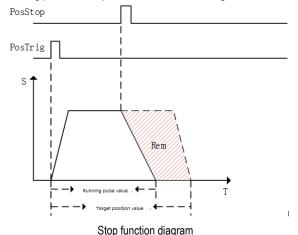
As shown in the figure above, the current running position command value is stopped by PosStop
