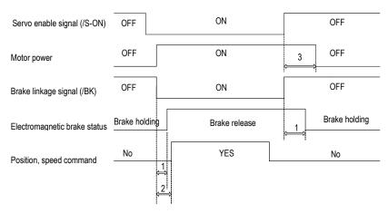
1. Different types of brakes may have slight difference on the time of holding brakes and loosening brakes.
